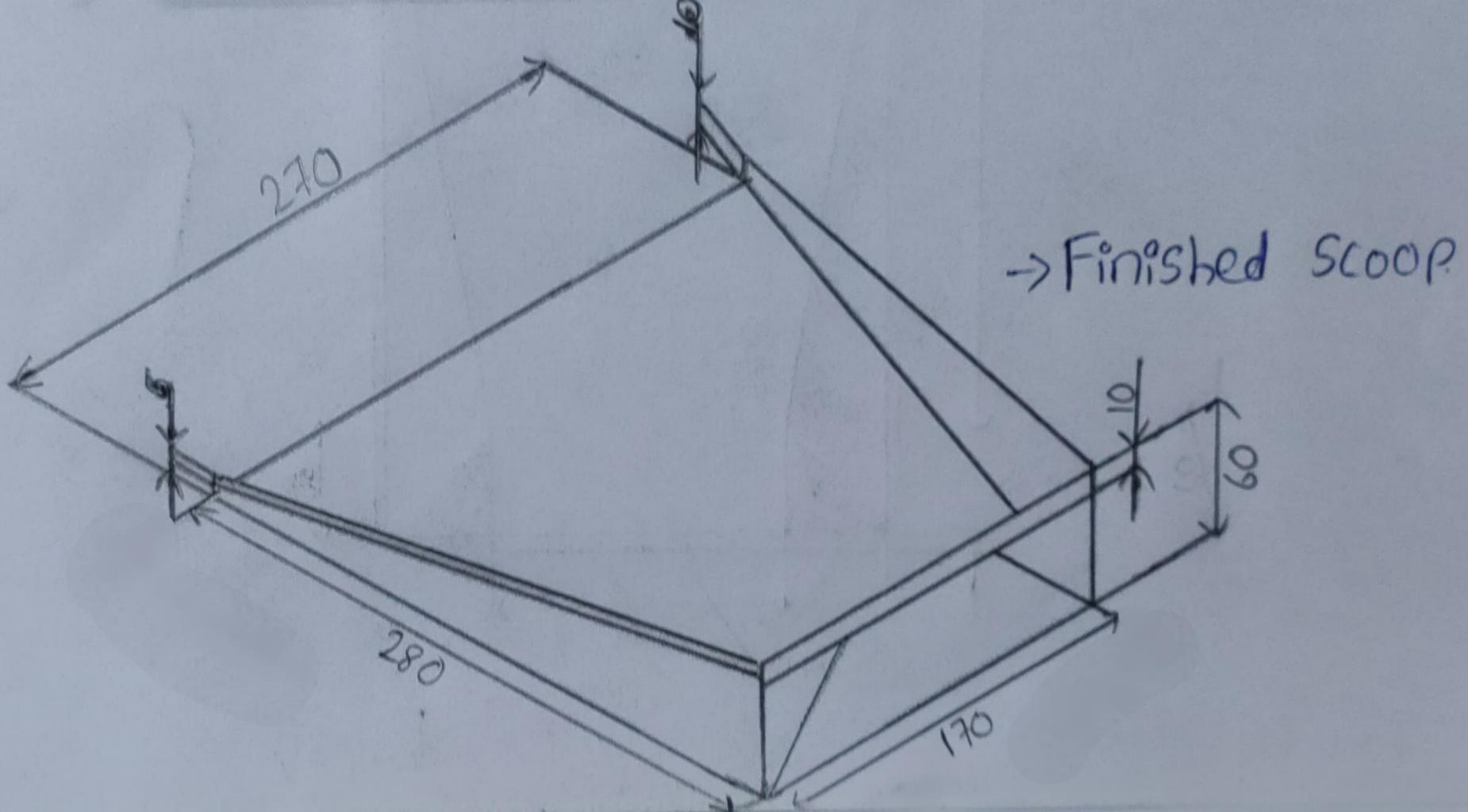
Aim :- To make a big scoop of given specification from a sheet metal piece.
