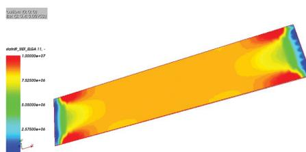
Figure 5 - PVB laminate, relaxation time 160s: Pattern of longitudinal axial SXX stresses
