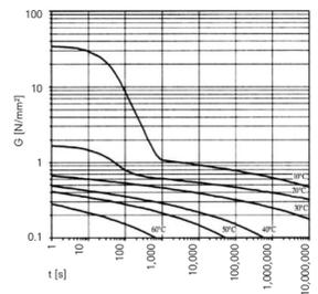
Figure 2 - PVB shear modulus in function of time and temperature [3]
