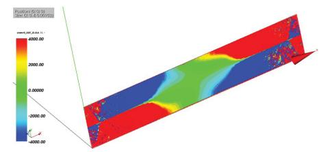
Figure 6 - PVB laminate, relaxation time 160s: Pattern of planar SXY shear stresses
