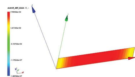
Figure 8 - PVB laminate, relaxation time 160s: Pattern of planar SXY shear stresses in the extrados
