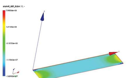
Figure 7 - PVB laminate, relaxation time 160s: Pattern of longitudinal axial SXX stresses in the intrados
