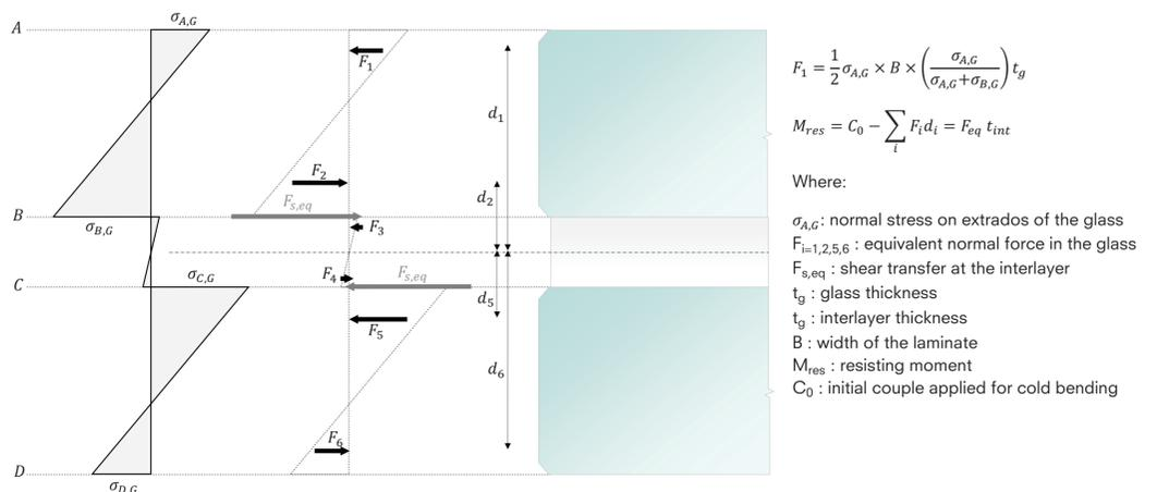
Figure 4 - Normal stresses at the face of glass and equivalent resisting moment in the interlayer
