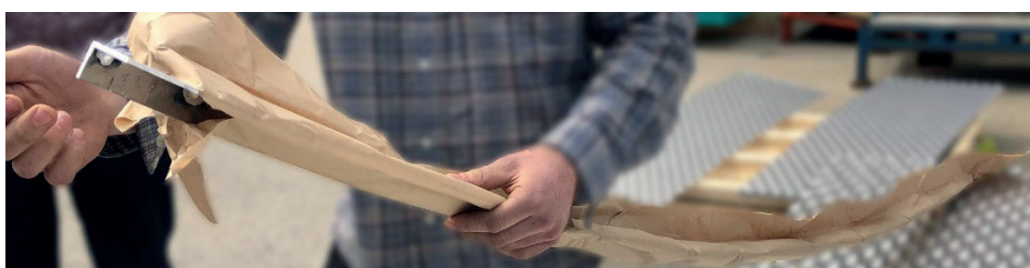
Figure 30: Welded curved aluminum V profile (undisclosed Enclos subcontractor)
