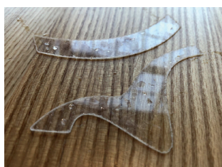
Figure 9,10,11: Waterjet cut laminated 0.1+0.1mm specimens
