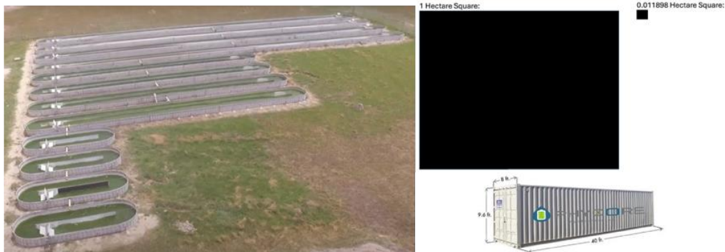
Example of a hectare phycoculture plant needed to decontaminate the Santiago Apostol swamp, compared to 0.011898 hectares that would be occupied by four compact reactors capable of doing the same work.
