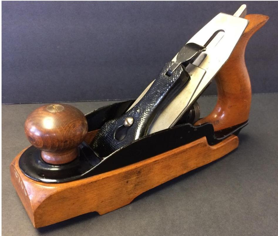
*Figure 1 Stanley prototype transitional furring plane*
