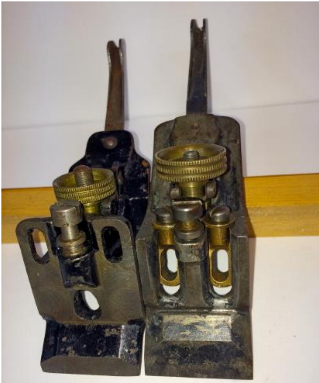
Figure 5 Under sides of Shaw's Patent frog (left) and prototype frog (right)
