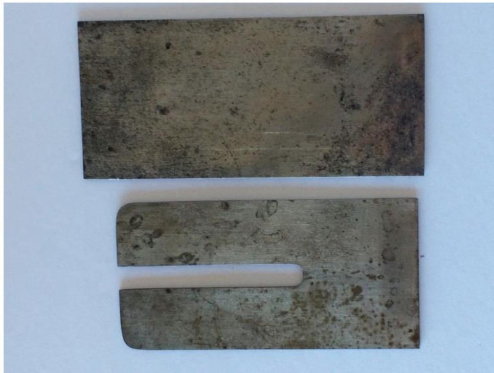
Figure 7 Production scraper cutter (top) and prototype scraper cutter (bottom)
