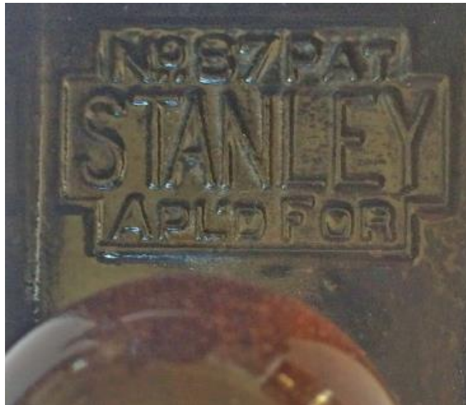
Figure 3 Detail of markings on body of production No. 87 scraper plane
