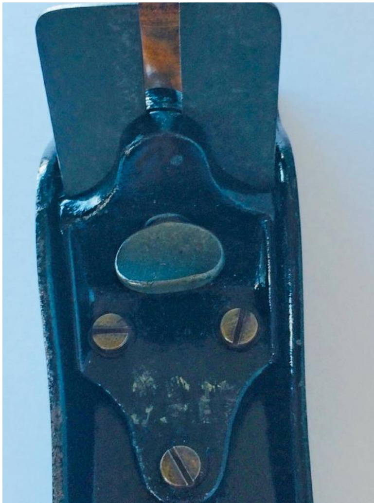
Figure 6 Detail of frog on prototype
