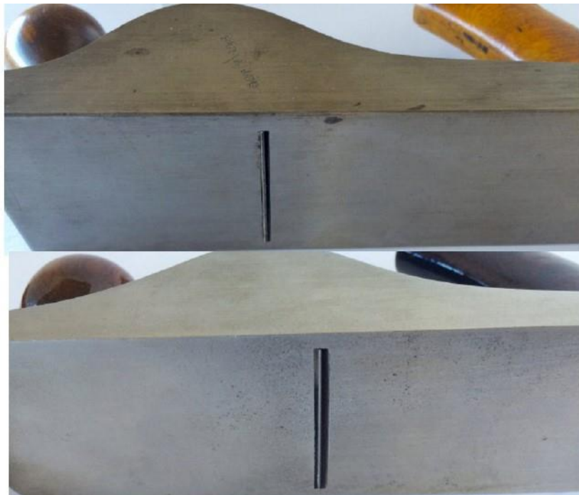
Figure 8 Mouth on prototype (top) and on production No. 87 (bottom)
