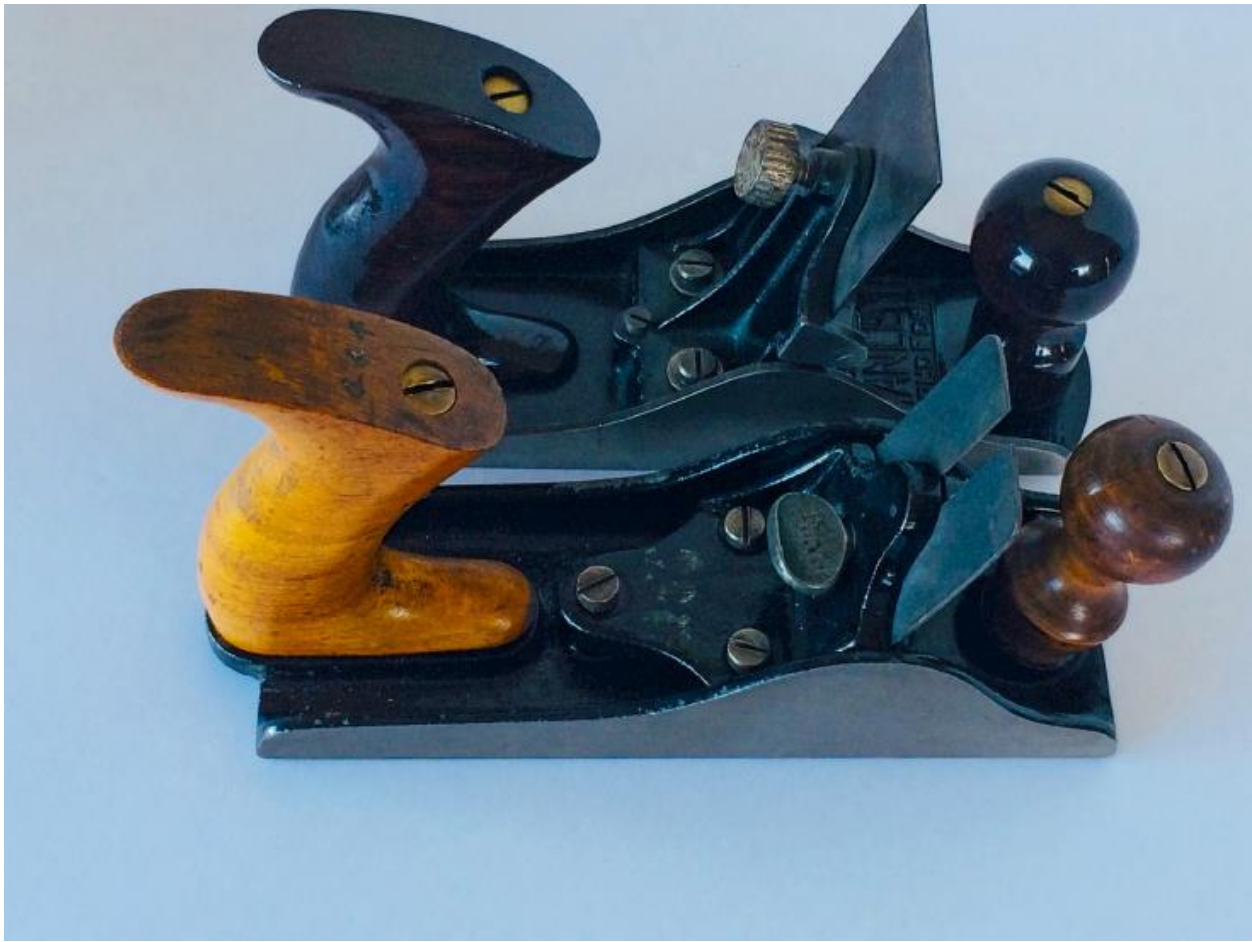
Figure 2 Comparison of the prototype (bottom) and production No. 87 scraper planes (top)
