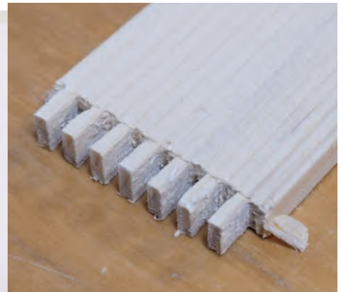
Finger Joint cuts made with Aubin Patent Saw
