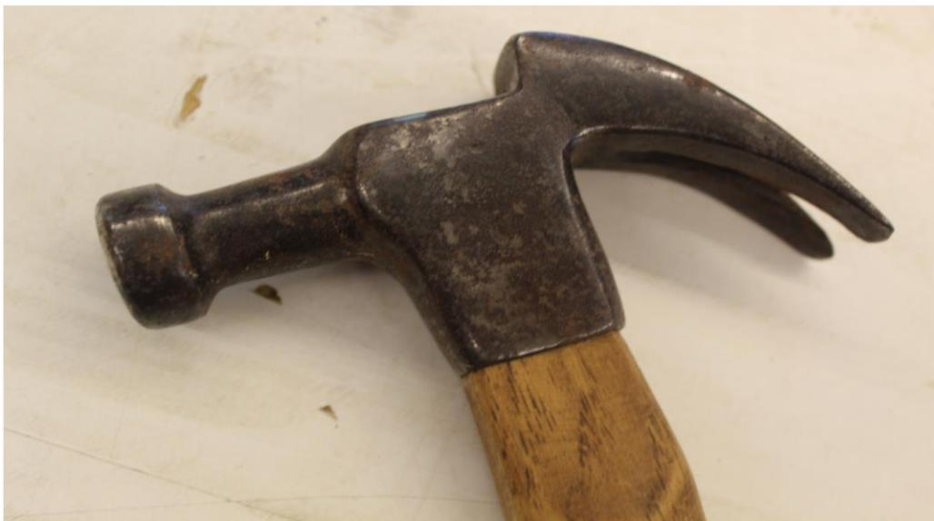
Hammer with offset fulcrum. From "The Hammer, the King of Tools" by Baird and Comerford.
