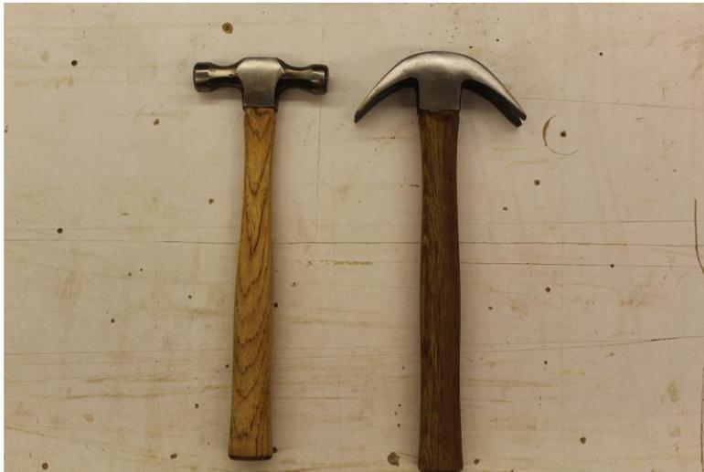
On the right: John Arrington patent wrecking hammer as shown in “The Hammer, the King of Tools” by Baird and Comerford. Conrad Berthold
