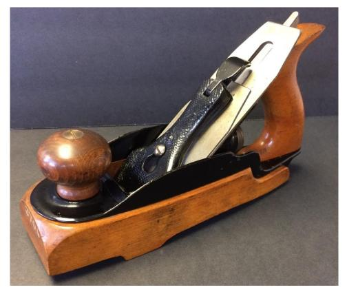
Figure 1 Stanley prototype transitional furring plane
