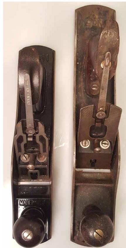
Figure 11: A No. 5-1/4 "Junior Jack" (left) alongside a standard No 5 (right), with the iron and chipbreakers removed.
