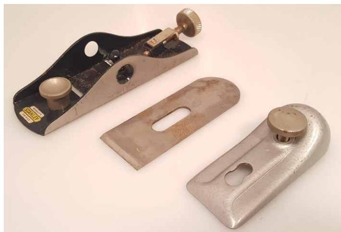
Figure 16. The No. 118 block plane body, blade, and lever cap (from left). This example is from 1960.
