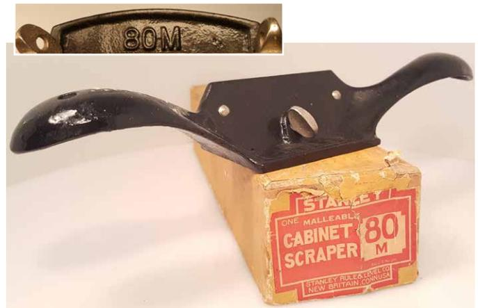
Figure 18. Stanley No. 80M cabinet scraper; inset: the top of the casting on the back.
