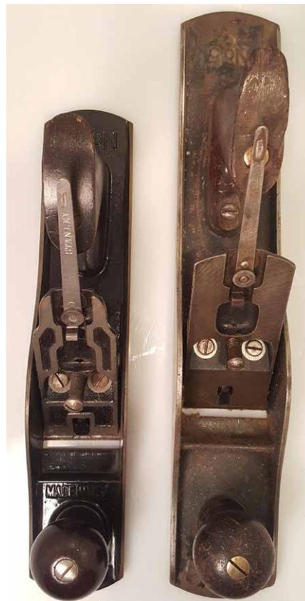
Figure 11: A No. 5-1/4 "Junior Jack" (left) alongside a standard No 5 (right), with the iron and chipbreakers removed.
