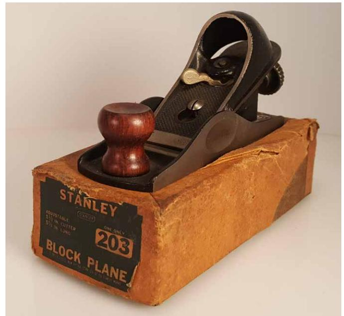
Figure 6. The Stanley No. 203 block plane was developed for industrial arts classes.
