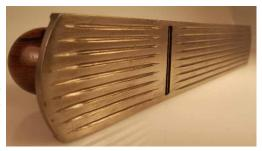
Figure 12. The corrugated sole of the Stanley No. 5-1/4C.
