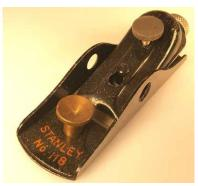
Figure 17. A 1940 example of the No. 118 block plane.
