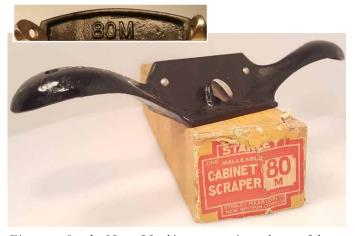
Figure 18. Stanley No. 80M cabinet scraper; inset: the top of the casting on the back.
