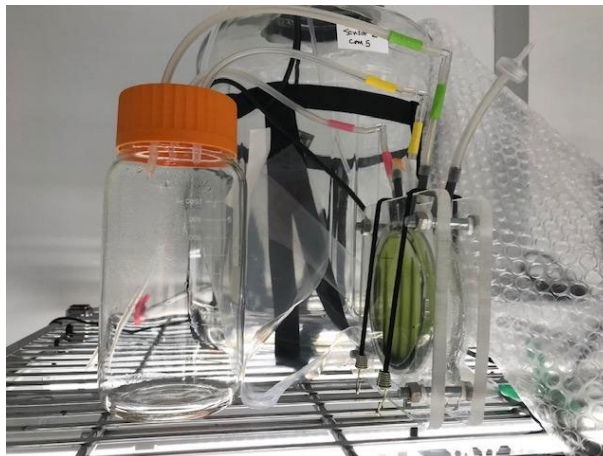
Fig. 8. Close-up of in-line filtration cassette. The 1-L bottle on the left was used for venting and overflow if the 1-micron membrane clogged. Cassette system designed by E. North. Photograph taken on 11/9/2019 by E. North.
