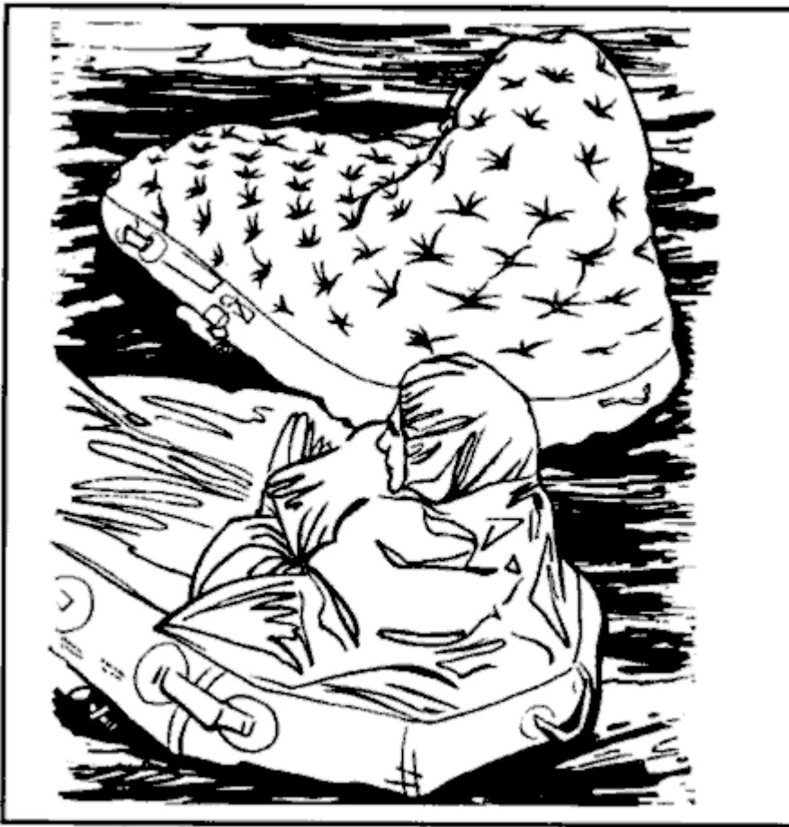
Figure 16-11. One-man raft with spray shield inflated.
