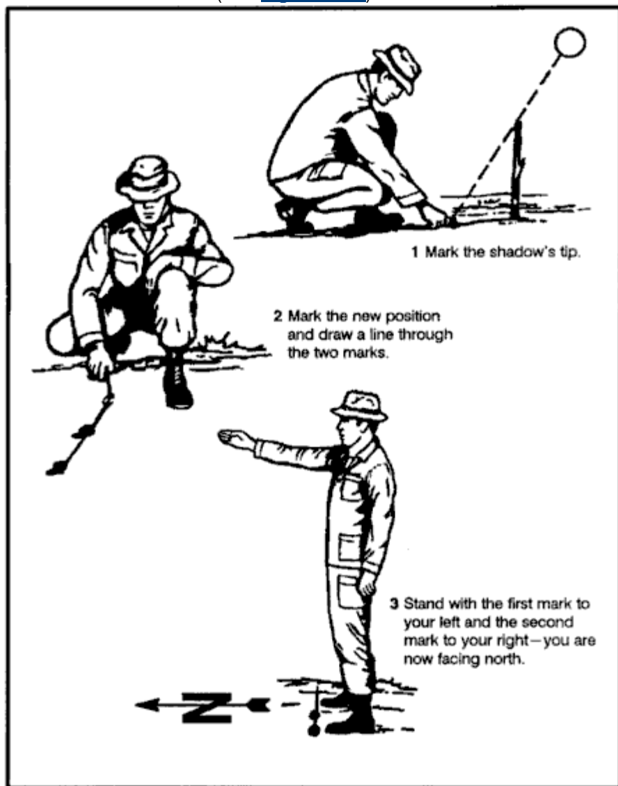
Figure 18-1. Shadow-tip method.
