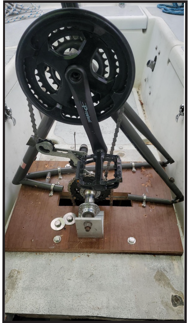
Peddle drive system made from old bike parts
