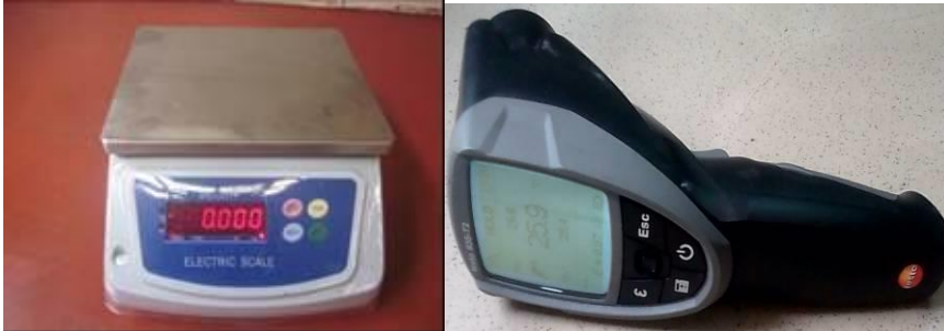
Figure 4: Auxiliary equipment used: Digital weighing scale and infrared thermometer
