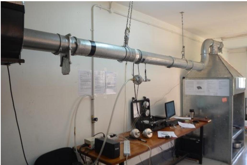
Figure 5: LEMS set up with the gravimetric system for emissions measurement PM2.5
