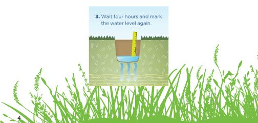
To determine the daily (24-hour) percolation, multiply the number of inches drained in four hours by six.
