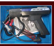
Cen-Tech Xenon Timing Light & Spark Plug Tester
