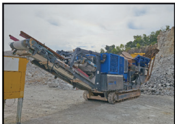
NX9161 '12 Kleemann MC 110 Z jaw crushing plant
