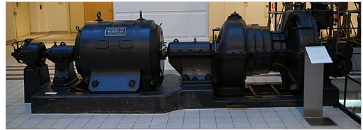
A 250 kW industrial steam turbine from 1910 (right) directly linked to a generator (left)
