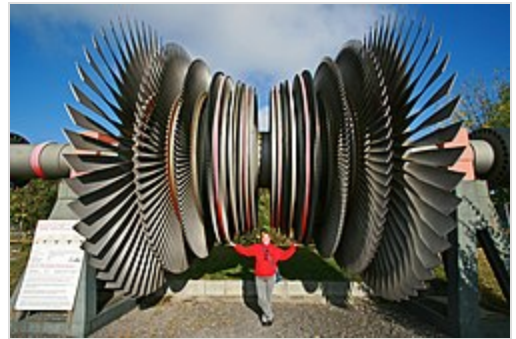
A two-flow turbine rotor. The steam enters in the middle of the shaft, and exits at each end, balancing the axial force.
