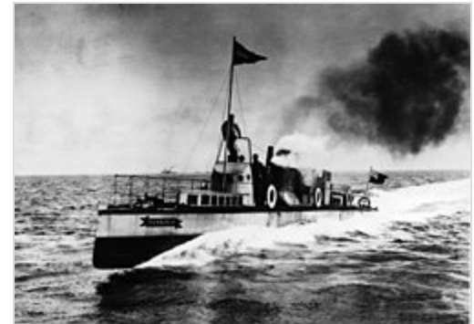
The first steam turbine-powered ship Turbinia : fastest in the world in 1894
