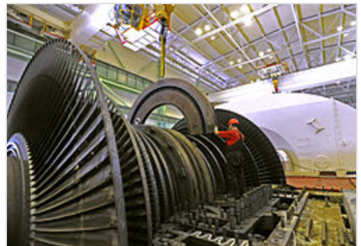
A low-pressure steam turbine in a nuclear power plant. These turbines exhaust steam at a pressure below atmospheric.
