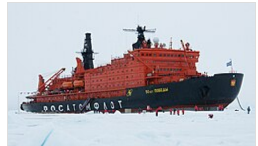
NS 50 Let Pobedy , a nuclear icebreaker with nuclear-turbo-electric propulsion
