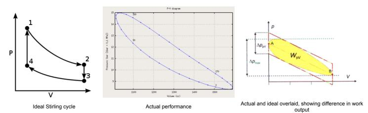
As the net work output for a cycle is represented by the interior of the cycle, there is a significant difference between the predicted work output of the ideal cycle and the actual work output shown by a real engine. It may also be observed that the real individual processes diverge from their idealized counterparts; e.g., isochoric expansion (process 1-2) occurs with some actual volume change.
