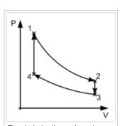
The clockwise thermodynamic cycle indicated by the arrows shows that the cycle represents a heat engine. The cycle consists of four states (the point shown by crosses) and four thermodynamic processes (lines).
