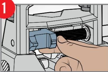
1 Select applicable Universal Press Block™ face and return block to center of push rod.
