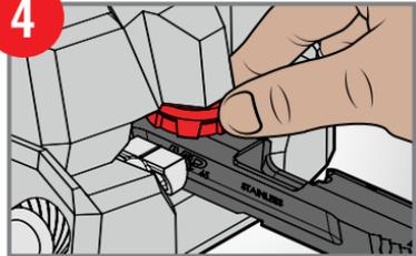
4 Snugly tighten vertical stabilizer to hold pistol slide in place.
