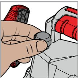
Turn both frame bolts simultaneously to avoid binding and keep upper frame level
