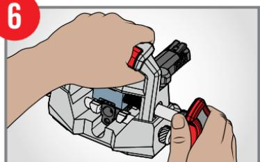
6 Turn Easy Torque Handle™ and push sight through dovetail slot.
