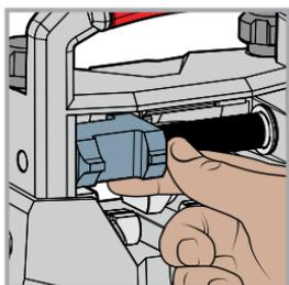
Select appropriate Universal Press block orientation. If you would like to use the opposite surface on the Press Block, rotate the crank clockwise to transport the Press Block all the way to the left. At this point, the pusher block should rotate freely without the support wall behind it. With the correct side selected, return the Press Block to the center by rotating the Easy Torque Handle counter-clockwise.
