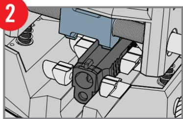
2 Align clamp guidelines with center of dovetail and secure slide in cradle.
