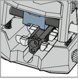
Loosen the two vertical frame bolts to allow for height clearance and help with visibility. Be sure to check the Hold Down Screw, to make sure it is up all the way. Mount pistol slide into slide frame.
