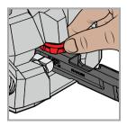
Once upper frame is moved to the correct position lower the Vertical Support Screw to the top surface of the slide to completely lock into place prior to pushing sight.
