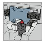
Use this step to ensure everything has remained aligned during the locking process and that the press block remains in correct alignment with the sight or dovetail slot and completely clears the slide to prevent damage.
