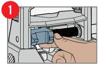
Select applicable Universal Press Block™ face and return block to center of push rod.
