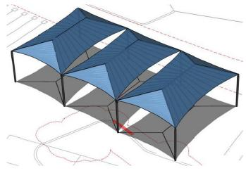
**Joined Four Post Hip Fabric Shade Structure** PC Model# DSA401J3040-19
