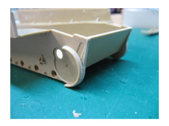
Simply trim off the front extension and sand flat with the front hull.
