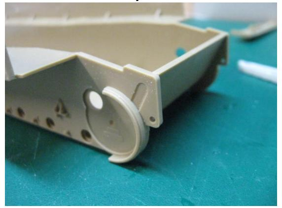
No need to fix this on the Rye Field Model or Dragon kits. The hull tub is the same on Tamiya Kit 35216 and there is no need to correct this if you are modelling Tiger 131
