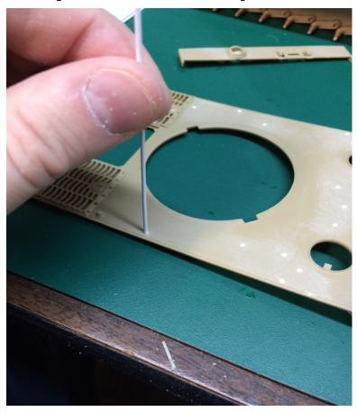
I used Evergreen .60 round styrene rod trimmed to fit. Let dry overnight then trim and sand flat. Use putty as needed.
