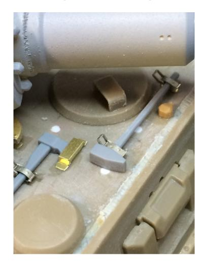
One thing I noticed when adding the shovel is that it can interere with the turret. The shovel and its clamps should be clear of the turrets ability to rotate.
