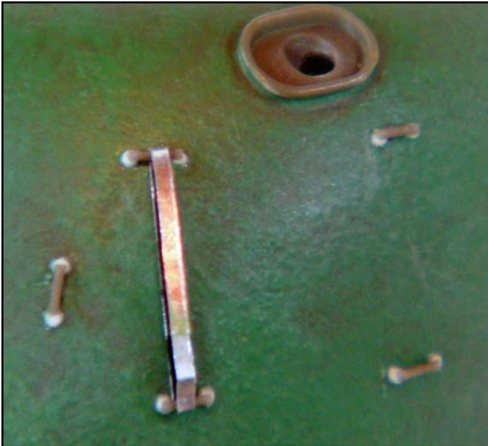
Here is a photo of several footman loops on a Sherman V turret. Note that these loops are formed using stretched sprue. The heavy foil strap illustrates how these loops can be used to actually attach items per the prototype.
