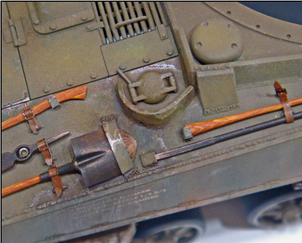
The final step is to add a small drop of supper glue on the "tail" of the strap under the point where the buckle will be, then hold the buckle end down (using a toothpick to avoid scratching the paint). After the glue sets, the strap paint can be touched up using a lighter shade of the base color for highlights.
