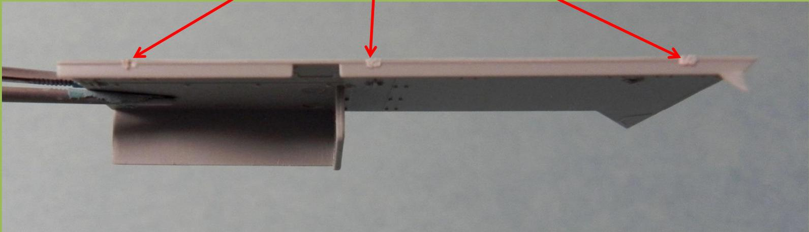
The sprue attachments cover the top edge of the armor plate and extend to the horizontal brace, making it hard to remove while maintaining the small step between the two.
