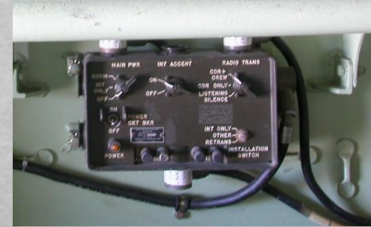
Master Intercom Control Box
