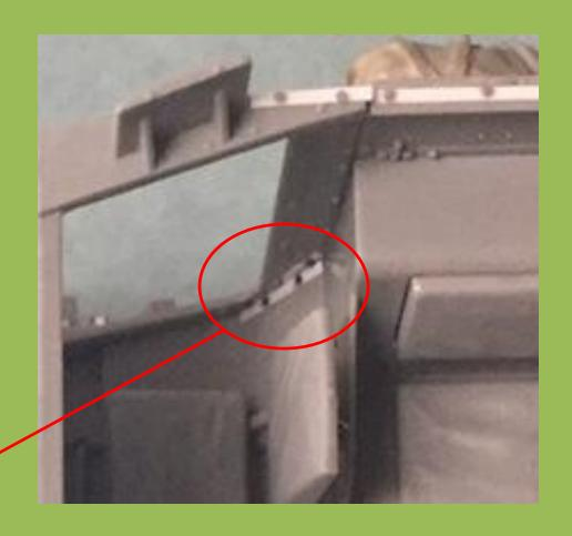
Mounting brackets added from 0.010" X 0.030" strip stock and 0.018" punched bolt heads.
