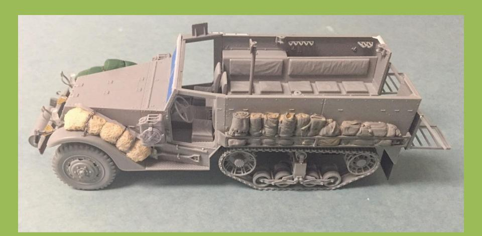
The cheese cloth was wetted down after rolling to rough shape and before fitting to the fender. It was formed to shape then white glue was dabbed on with a disposable brush to harden.
