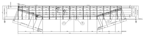
Structural Dip Tank Engineering, Design & Detailing
