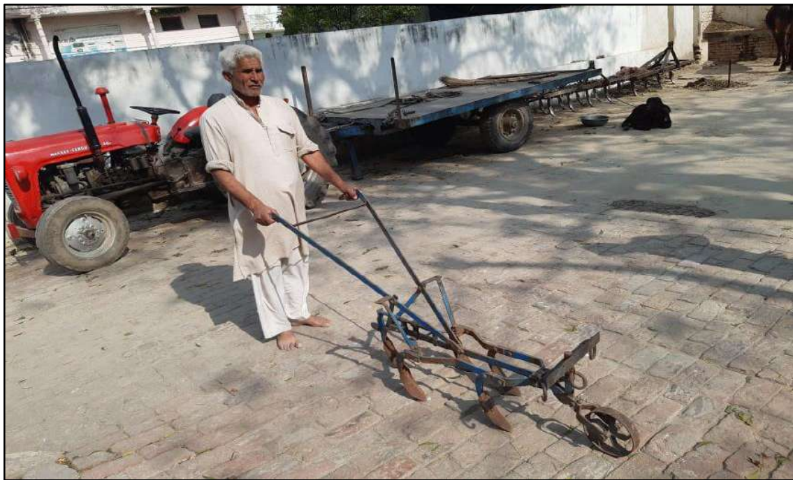
Fig 7. Animal drawn cultivator used in sugarcane for weeding and intercultural operation
