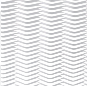
MODEL: HJAX-10012 Thickness=2.0mm Strand width=2.0mm SWDxLWD=12x100mm Open area=65%
