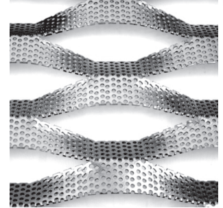
MODEL: HJAX-80200 Thickness=3.0mm Strand width=29mm SWDxLWD=80x200mm Open area=54%
