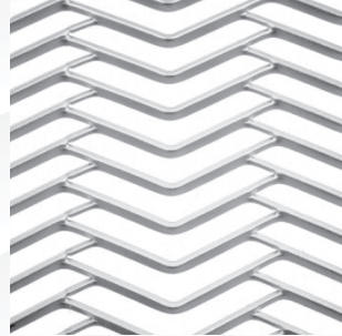
MODEL: HJAX-12100 Thickness=3.0mm Strand width=3.6mm SWDxLWD=12x100mm Open area=38%
