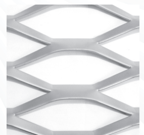
MODEL: HJAL-45155 Thickness=3.0mm Strand width=10mm SWDxLWD=45x155mm Open area=52%
