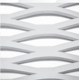
MODEL: HJAL-34135 Thickness=5.0mm Strand width=10mm SWDxLWD=34x135mm Open area=40%
