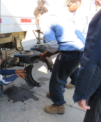
Pictured above; Student Jalen Neal installs new rear brake shoes on a trailer belonging to the center.
