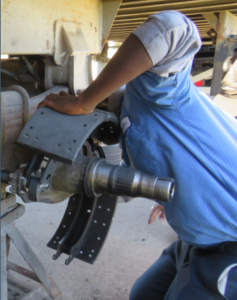
Pictured above; Student Jalen Neal installs new rear brake shoes on a trailer belonging to the center.
