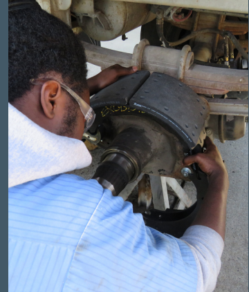
Pictured above; Student Jalen Neal installs new rear brake shoes on a trailer belonging to the center.
