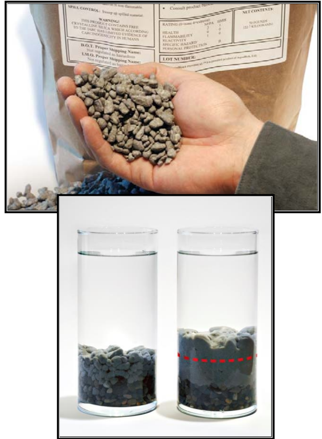
Figure 1. Configuration of stone-clay composite particle.
