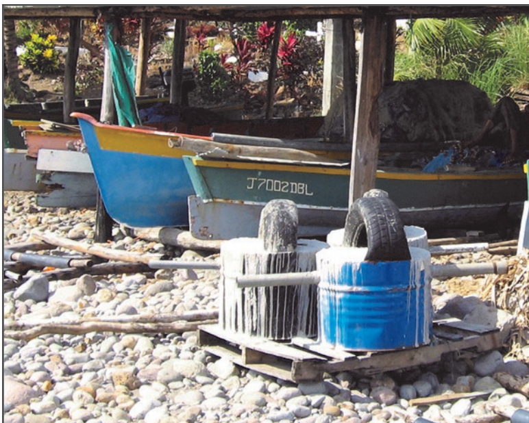
Figure 18: FAD anchors at Dublanc
