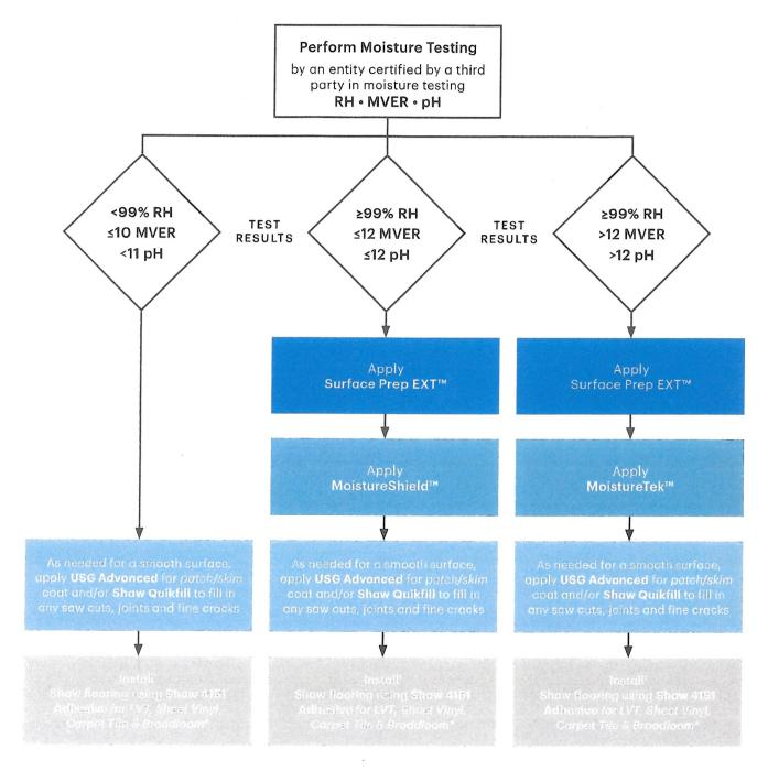
MVER - Moisture Vapor Emission Rate, measured by the Calcium Chloride Test
