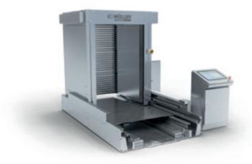
For hygienic reasons, goods entering on wooden pallets often need repalletizing – on aluminum, plastic or clean wood pallets. Manual and automatic Müller pallet changers ensure easy and safe handling of the load.
