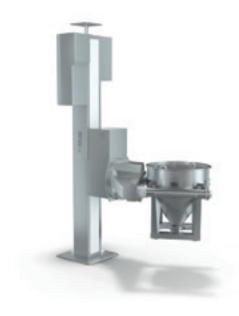
Müller drum and container blenders guarantee the precise and safe carrying of blending containers of varying sizes. The recipe management allows optimal adaptation of the product to be blended. The facilities offer high blending performance for a wide range of powders while preserving substance quality.
