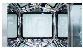
The washing chambers of the GMP washers offer low ultrapure water consumption and efficient and reliably reproducible clean and drying processes.
