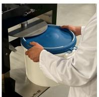
2. Slide the container into the closing machine until it reaches the rubber stops.
