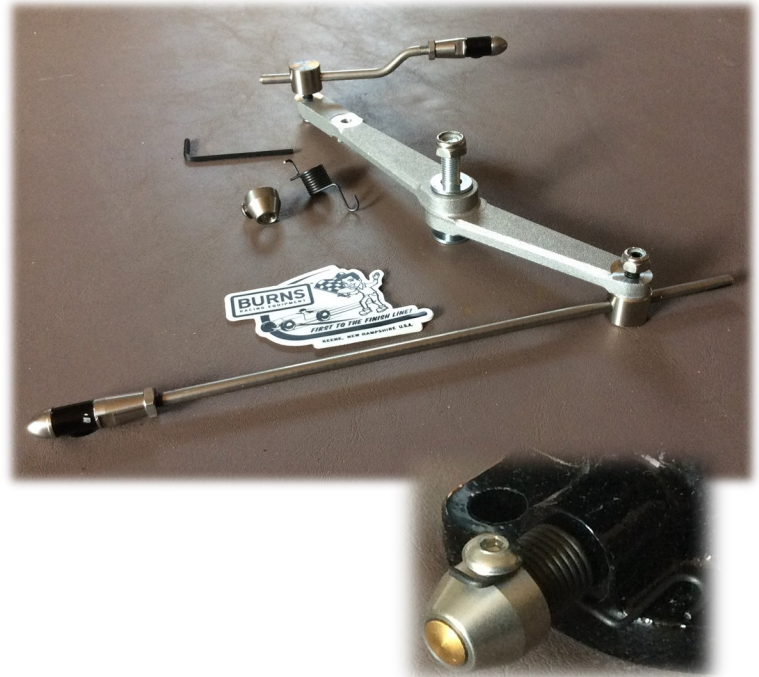
Detail - Throttle Return Set-Up on Single Carb Linkage
