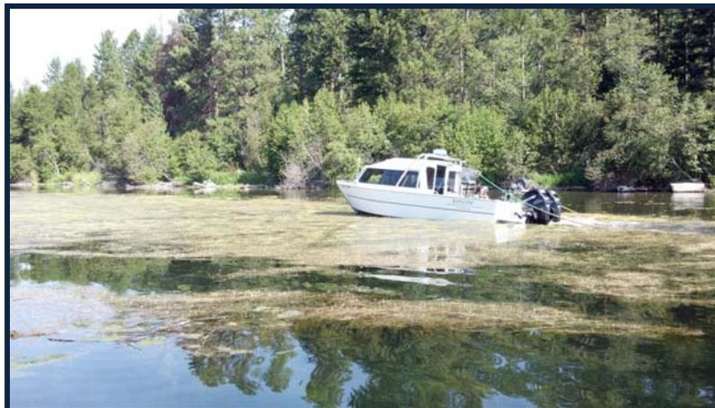
The AIS treatment area GIS shapefiles were loaded into the LittLine<sup>®</sup> computer system's for vessel guidance and herbicide application data recording. The treatment tracks were automatically recorded via the LittLine vessel's GPS guidance system for the production of the final treatment area maps to document the treatment areas.
