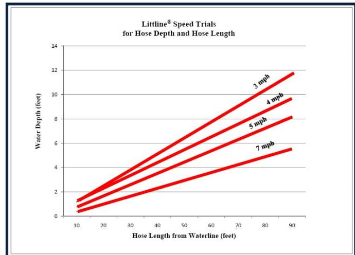
to support the LittLine<sup>®</sup> vessel operator adjust speed based on water depth in a specific treatment Plot (chart shown to the right, Speed Trials performed in Lake Coeur d'Alene, September 8, 2009, independent third party depth data collected by Jim Flodin, Divers West, CDA Idaho). The LittLine<sup>®</sup> hoses are electronically reeled in or reeled out based on the varying depths of the treatment Plots.
