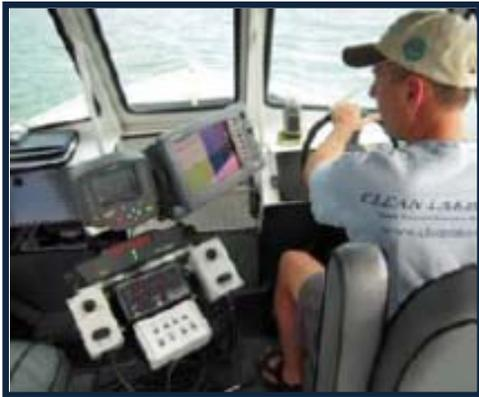
through preset treatment rates. When the vessel speeds up and or slows down, the rate controllers adjust the herbicide application rate to match the preset rate in gallons of product per acre.
