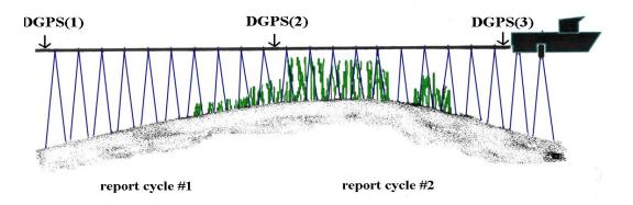
The sonar data collected was processed and analyzed for At Time of Treatment Submerged Aquatic Vegetation (SAV) in the treatment plots and at ~ 6 Weeks Post Treatment. Data was collected to compare At Time of Treatment and ~ 6 Weeks Post Treatment SAV coverage, height in the water column, and biovolume to support post-treatment efficacy evaluations. An example of SAV conditions at time of treatment for Plot C-3-14, Cabinet Gorge Reservoir, is pictured to the right.
