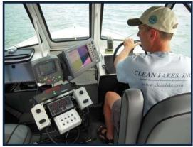
The LittLine system's computerized rate controllers regulate the aquatic herbicide applications through preset treatment rates. When the vessel speeds up and or slows down, the rate controllers adjust the herbicide application rate to match the preset rate in gallons of product per acre.
