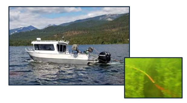
The AIS treatment area GIS shapefiles were loaded into the LittLine<sup>®</sup> computer system for vessel guidance and herbicide application data recording. The LittLine<sup>®</sup> can place herbicides at any depth within the water column (2 - 30 feet), as well as within the bottom 2 foot of the water
