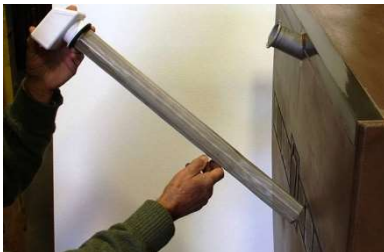
Additive Sleeve for Oak Alternatives (Chips, Rice, Beans)
