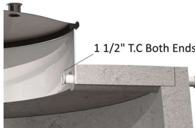
Pump-over Tube Embedded
