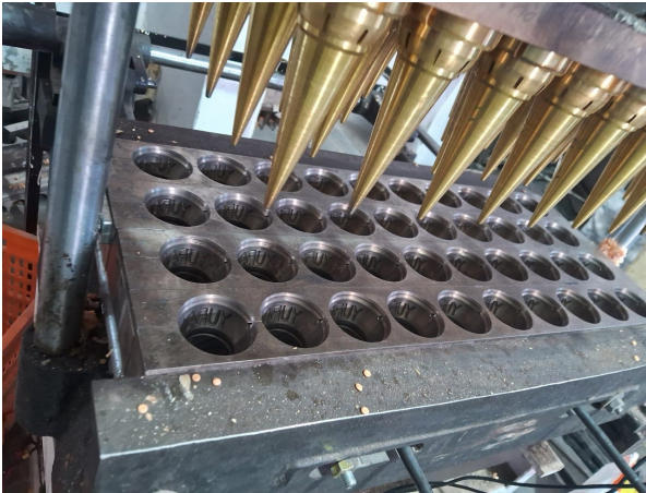
Cone machine forming dies in operation
