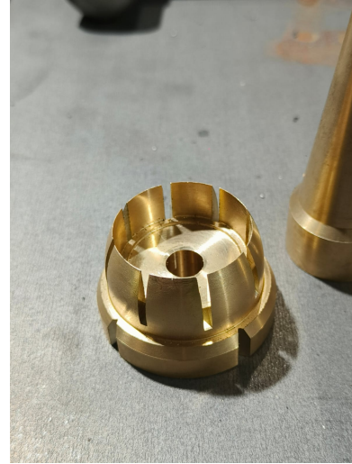
Machined brass die with slotted cavity
