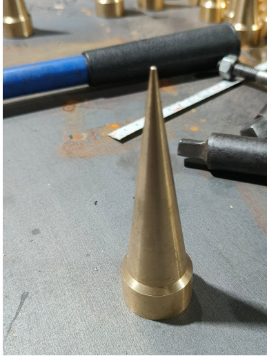
CNC-turned brass forming cone
