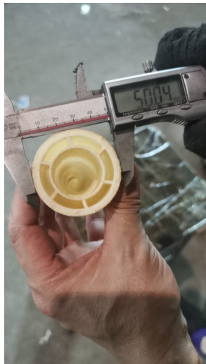
Cavity diameter verification
