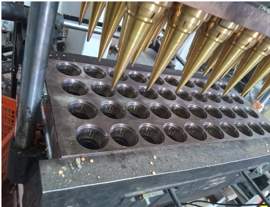
Multi-cavity brass forming dies producing precision wafer cones
