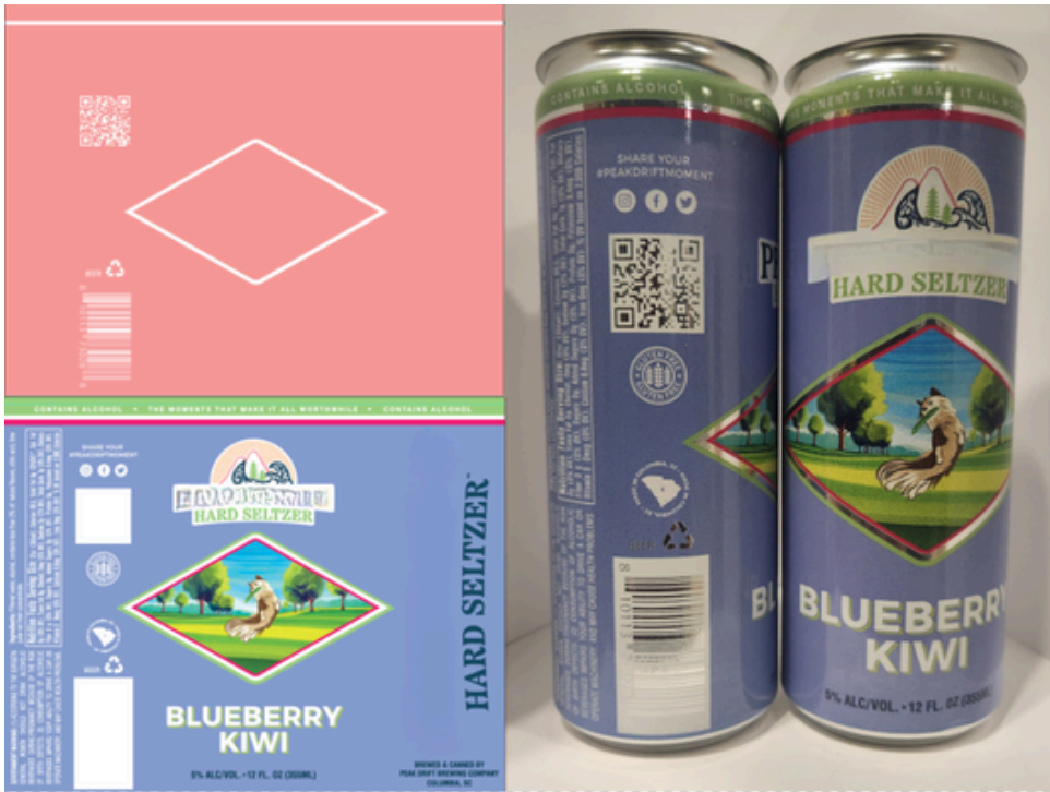
*This example shows how Spot Color (White Underlay) can be removed from the "White Underlay" layer to create a "knockout" in printed design. This allows the aluminum of the can to "knockout" through the printed design. Below the "White Underlay" layer , you'll see the "Artwork" layer . Notice there is white in the artwork, but it doesn't print? This is due to the Spot Color (White Underlay) /pink color being removed in the "White Underlay" layer . IF there was another color other than white in the "Artwork" layer , that color will print over the aluminum (without a white background printed) creating a metallic color finish . Example below.
