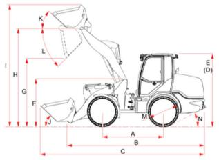
A. 48.4 IN H. 85.4IN B. 87 IN I. 117.3 IN C. 114.2 IN J. 43 DEGREES D. 81.1 IN K. 43 DEGREES E. N/A L. 46 DEGREES F. 55.5 IN M. 22.4 IN G. 54.3 IN N. 34 DEGREES
