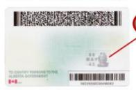
Laser- engraved image with tilting effect incorporated in plastic cards: images are engraved at different angles through an array of cylindrical lenses embossed into the surface of the card. Angle of view effects a change.
